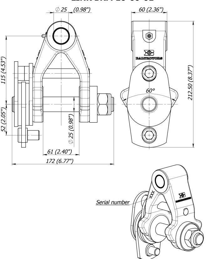
\* Pin locking nut is tightened with a torque of 60 - 160 Nm (45 - 120 lb ft) dependent on desired brake power. \* Weight - 5 kg (11 lb) \* Fill grease Starplex EP 2, through lubricating nipple (pos. 12), until it will appear to the external surfaces. Greasing must be repeated after every 8 working hours of the link.
